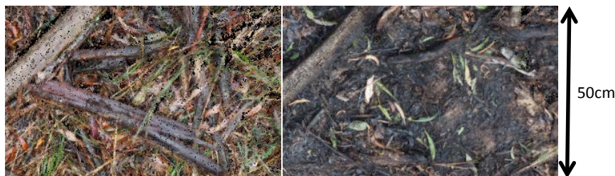
Figure 2. a) pre and b) post - burn orthophoto (generated at 2 mm resolution) generated from fuels3D data capture.
