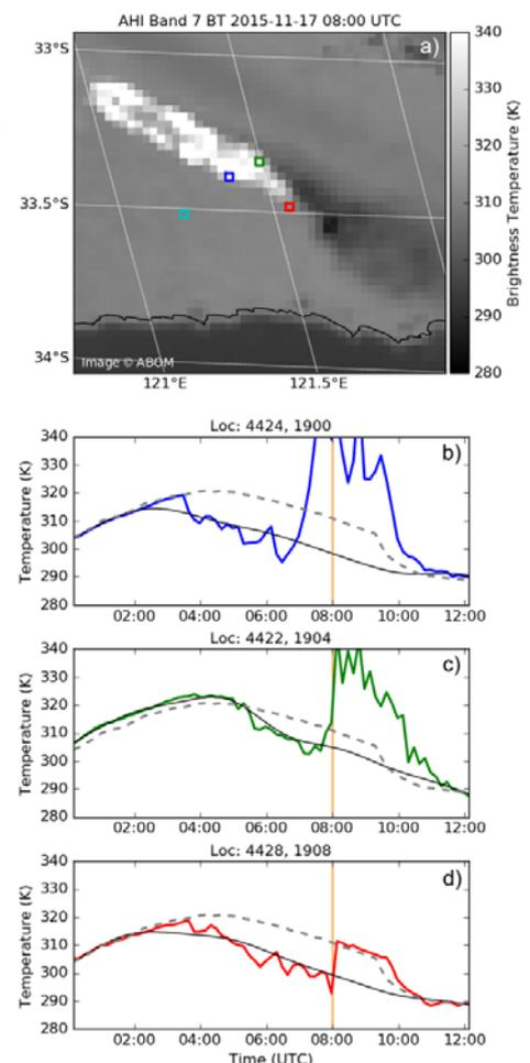
Figure 1. a) brightness temperatures from the medium wave infrared band 7 of AHI, 1600 AWST. b, c, d) coloured line = raw brightness temperatures of selected pixels, black line = SVD fitting of DTC, dotted line = sample brightness temperature of pixel at [4429,1894] shown in cyan on Figure 1a, orange line = time of AHI image in Figure 1a.
