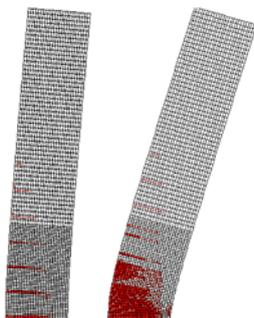
In light of these recent observations, there is a need to investigate the amount of longitudinal reinforcement required to initiate secondary cracking and allow a distribution of plasticity. These results are essential knowledge for vulnerability studies of reinforced concrete buildings that are being carried out by the authors within the earthquake mitigation component of the Australian Bushfire and Natural Hazards Cooperative Research Centre.
