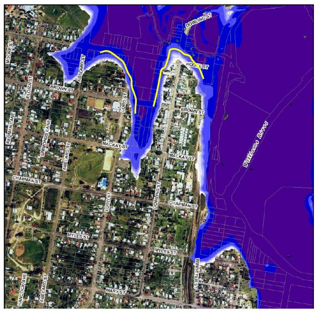
Figure 2.7 Extract from BMT WBM (2009) showing modelled flood extents for the Probable Maximum Flood Event. The yellow lines superimposed on the images represent the high water level for the 20-21 April, 2015 event derived from field observations, interviews with residents and photos supplied by Dungog residents.
