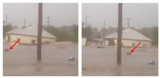
Figure 4.11 Two stills taken from Youtube (2015) at 31 seconds and 34 seconds after commencement of the video. The two stills show where the debris item, arrowed, crosses sight lines between the camera and power poles.
