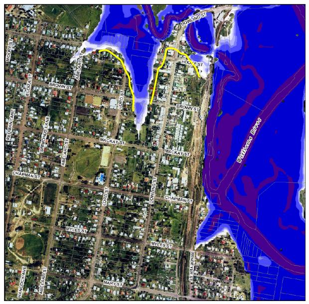
Figure 2.6 Extract from BMT WBM (2009) showing modelled flood extents for the 0.5% AEP Flood Event. The yellow lines superimposed on the images represent the high water level for the 20-21 April, 2015 event derived from field observations, interviews with residents and photos supplied by Dungog residents.
