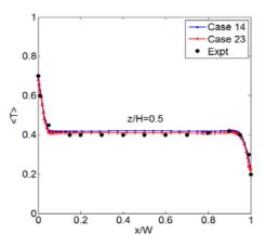
Figure 10. A Computed and measured temperature profiles at the mid-height of a differentially heated cavity.
