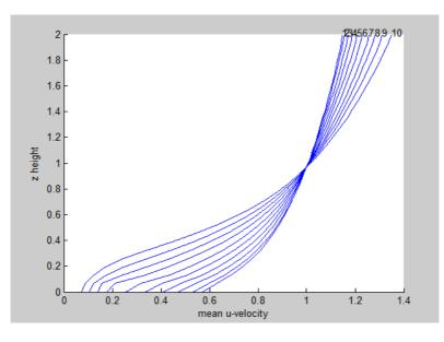
Figure 2: Mean centreline u-velocity profile over the canopy for a 1/7-power law input profile. (1) is in the canopy-free region, and (10) is at the end of the canopy. Note the velocity profile has been normalised by the velocity at the top of the canopy, and the results is preliminary.
