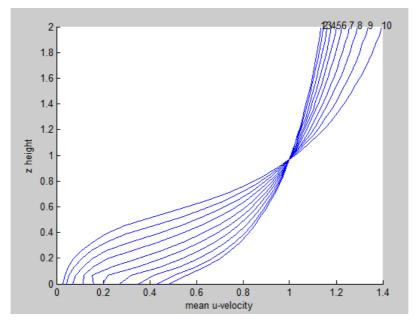
Figure 1: Mean centreline u-velocity profile over the canopy for a logarithmic input profile. (1) is in the canopy-free region, and (10) is at the end of the canopy. Note the velocity profile has been normalised by the velocity at the top of the canopy, and these results are preliminary.
