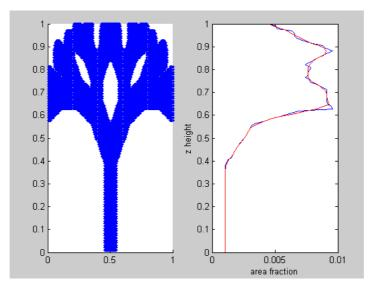
Figure 4: The same example fractal tree as in figure 3, but blurred by a Gaussian filter, and corresponding A(z) (blue) and smoothed A(z) (red).
