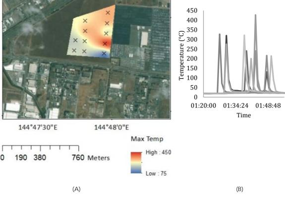
FIGURE 2 MAXIMUM TEMPERATURE RECORDED IN THE BURNED GRASSLAND AREA (A) AND TEMPERATURE REACHED BY EACH SENSOR OVER TIME (B).
