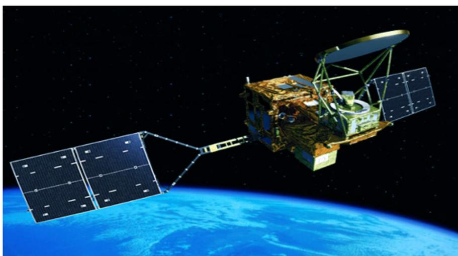
Fig 1: AMSR2 radiometer onboard G-COMW satellite
