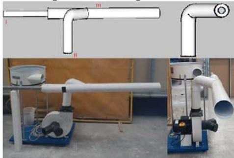
Fig. 2 Firebrand generator prototype front and side view
