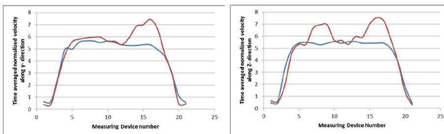
Fig. 3 (a) & (b) Simulated average velocity profile in two perpendicular directions (Y) and (Z) as shown in Fig. 1(b) — Extended design — Original design
