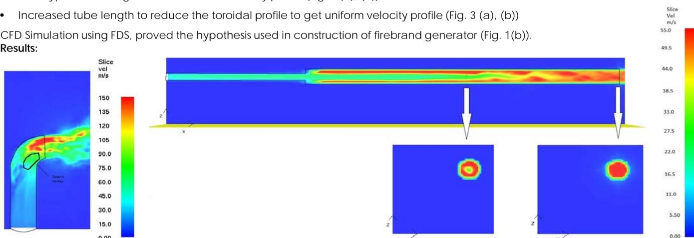
Fig. 1(a) & (b) CFD velocity profile for NIST firebrand dragon showing a low velocity region near the bend in the tube (Dean's vortex) and VU Firebrand generator showing the cross-sectional velocity profile becoming more uniform as the length of the outer tube increases.
