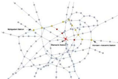
Figure 3: Rerouting of the shortest path (km) from Myogadani Station to Monzen-Nakacho Station after Otemachi Station was removed from the Tokyo Metro network. Original path in red, detour in yellow.
