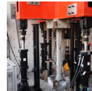
Testing of RC columns in Swinburne's state-of-the-art Smart Structures Laboratory
