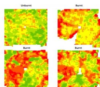
Figure 5. Maps derived from terrestrial laser scanning (see Figure 4) three months after a burn event showing areas of minimal to no change (green), small change (yellow) and large change (orange/red).
