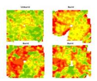
Figure 5. Maps derived from terrestrial laser scanning (see Figure 4) three months after a burn event showing areas of minimal to no change(green), small change (yellow) and large change (orange/red).
