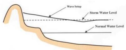
Figure 2. Illustration of the wave setup component of surge at a coast.
