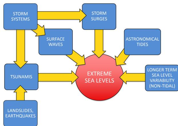
Figure 1. Illustration of the various physical processes that contribute to create extreme water levels.
