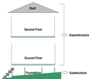
Figure 1. Building structure and main components
