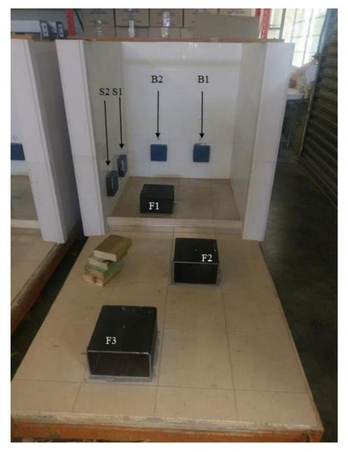
FIGURE 8: LOCATION OF TILES TO BE TESTED AND ANHOR POINTS BONDED ON TILES
