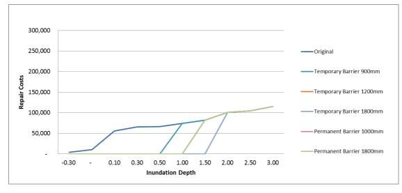
FIGURE 15: VULNERABILITY CURVES FOR STOREY TYPE 2 - ORIGINAL AND FLOOD BARRIERS
