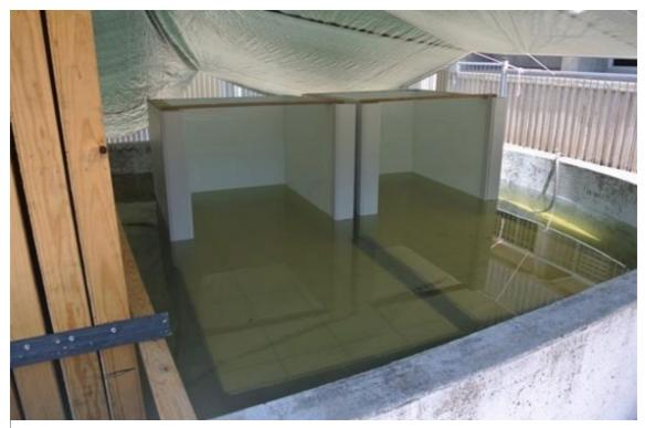
FIGURE 7: BATHROOM SAMPLES IN WATER TANK DURING FLOOD SIMULATION
