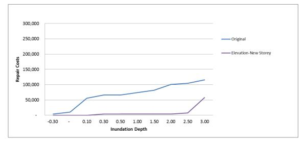
FIGURE 13: VULNERABILITY CURVES FOR STOREY TYPE 2 – ORIGINAL AND ELEVATED (NEW STOREY)
