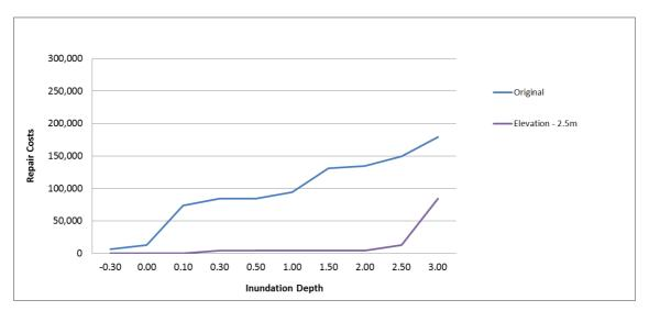
FIGURE 11: VULNERABILITY CURVES FOR STOREY TYPE 1 - ORIGINAL AND ELEVATED
