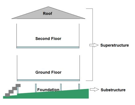
FIGURE 2: BUILDING STRUCTURE DIVIDED INTO MAIN COMPONENTS
