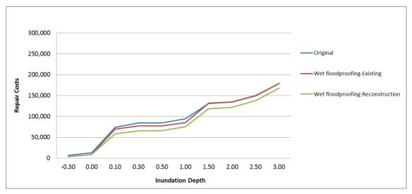
FIGURE 12: VULNERABILITY CURVES FOR STOREY TYPE 1 - ORIGINAL AND WET FLOODPROOFED
