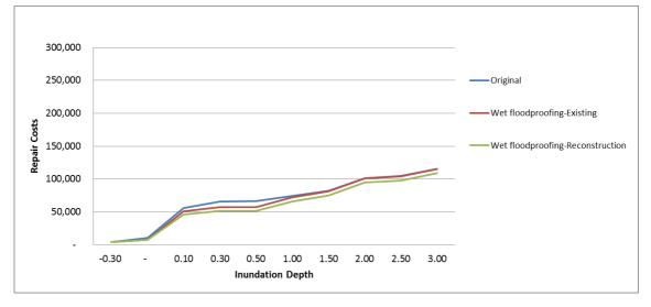
FIGURE 14: VULNERABILITY CURVES FOR STOREY TYPE 2 - ORIGINAL AND WET FLOODPROOFED
