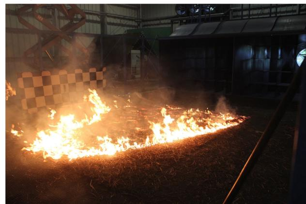
Above: Final stages of a rate of spread experiment with a line fire conducted on a flat fuel bed
