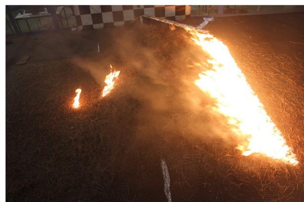
Above: Rate of spread experiment with a line fire spreading up a model hill towards two manually ignited spot fires on the lee side of the hill.
