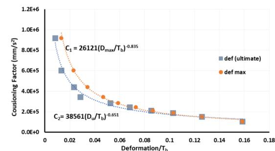
Fig. 4: Cushioning factor's relationship with the beam deformation
