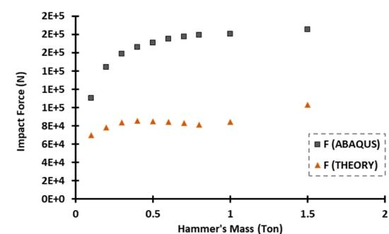
Fig. 3: Normalised maximum impact force relationship with the normalised maximum mass of the impactor
