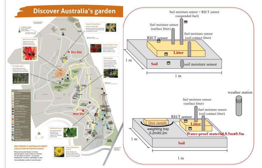
Fig. 1. The two experiment sites on the visitor map (left), and the parallel experiments and instruments at each site (right).
