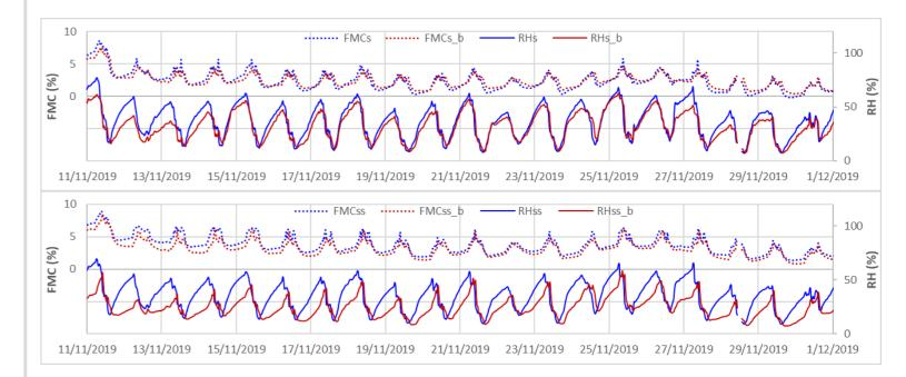
Fig. 2. Time series of FMC and RH at the dry site. FMC<sub>s</sub>, RH<sub>s</sub> and FMC<sub>s</sub>, RH<sub>ss</sub> represent FMC and RH in surface and subsurface litter, respectively, for the treatment without the barrier. FMC<sub>s b</sub>, RH<sub>s b</sub> and FMC<sub>ss b</sub>, RH<sub>ss b</sub> represent FMC and RH in surface and subsurface litter, respectively, for the treatment with the barrier.
