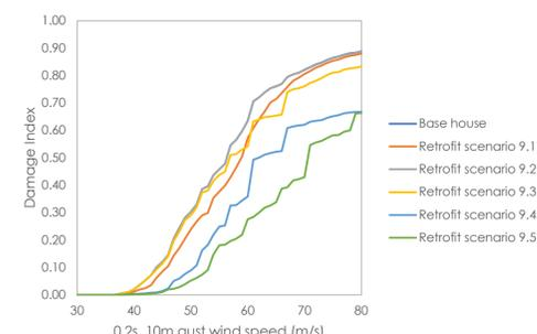
Figure 2 Vulnerability functions for house type 9 – brick veneer + metal roof cladding
