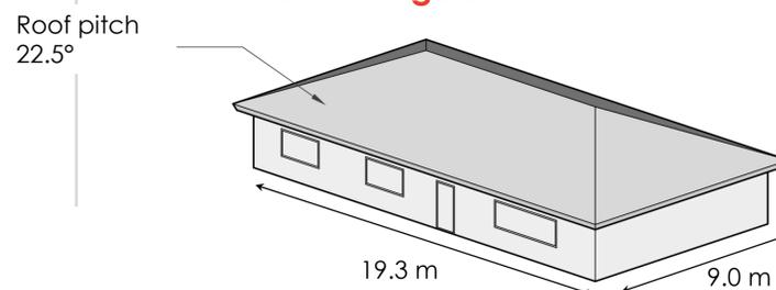
Figure 1 Overall dimensions of the hipped roof generic house types
