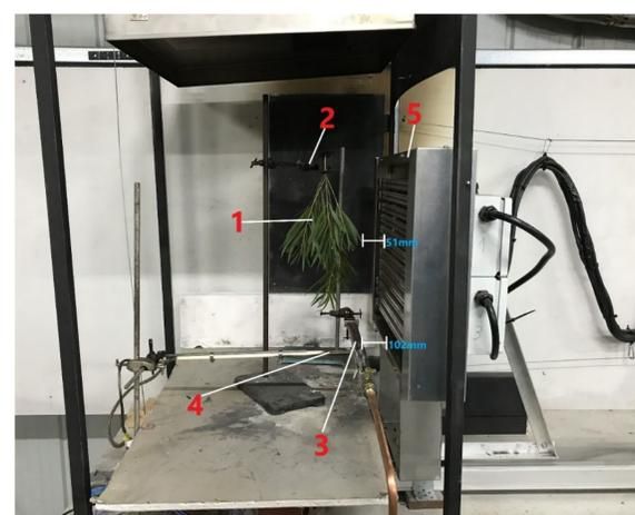
Figure 1: Experimental design: 1) sample, 2) clamp, 3) pilot igniter, 4) spark igniter, 5) radiative panel.
