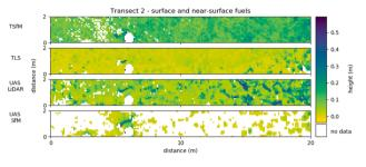
Fig. 4. Comparison of surface and near-surface fuel height in transect 2 between TSfM, TLS, UAS LiDAR and UAS SfM dervied point clouds.
