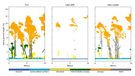
Fig. 6. Side view transect through a section of the study plot demonstrating the raster pouring classification of vegetation into canopy, stems intermediate canopy, elevated, surface/near-surface and ground layers.
