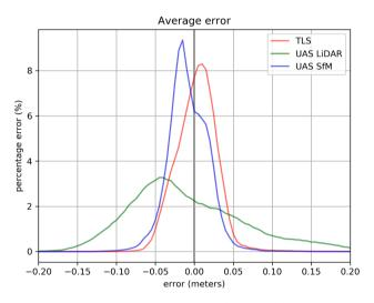
**Fig. 3.** Histograms showing the error between the terrestrial image based point cloud defined ground surface and the three other technologies.
