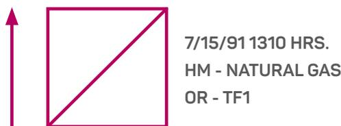
Figure 3: FEMA Structures and Hazards Marking (US Army 2016).
