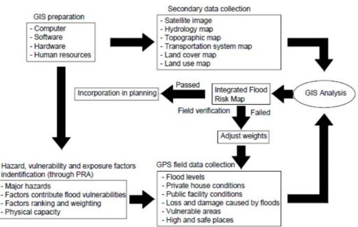
Figure 14 Flood risk mapping process
