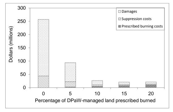
Figure 6.4. Damages, suppression costs and prescribed-burning costs for each prescribedburning rate applying the current strategy: long-term analysis
