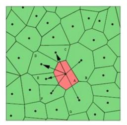
Figure 4.3. AUSTRALIS irregular cell grid
