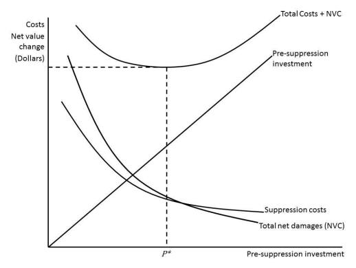
Figure 4.1. The cost plus net value change (C+NVC) model
