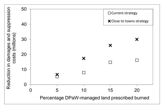
Figure 5.12. Reduction in damages and suppression costs for each strategy for different prescribed-burning rates
