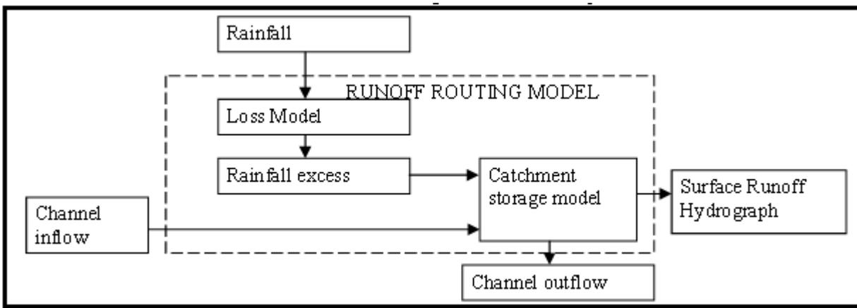
**Figure 3.9. Overall RORB Runoff Routing Model (Monash University, 2015)**
