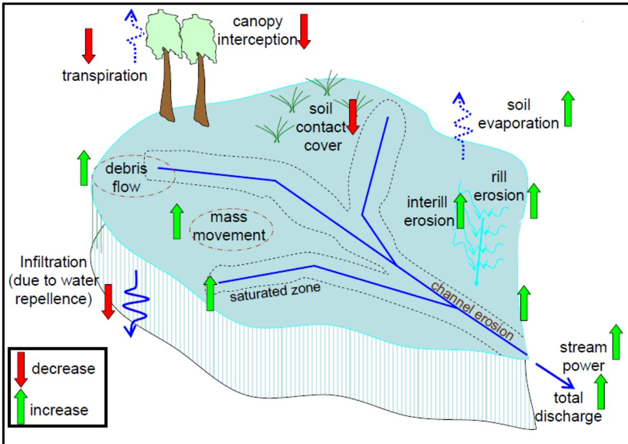
Figure 3.4. Schematic diagram showing possible post-fire changes in hydrologic and erosion processes (Smith et al., 2011a)
