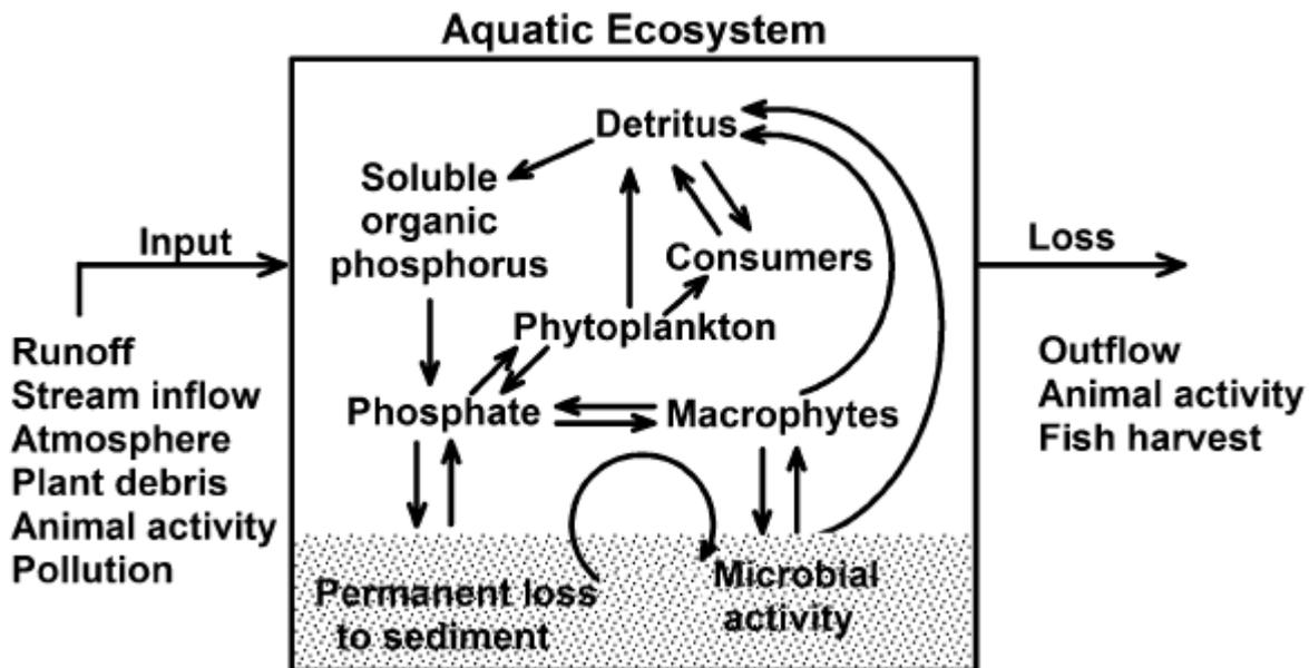
Figure 3.2. A qualitative model of the phosphorus cycle in an aquatic ecosystem (Boyd, 2015)
