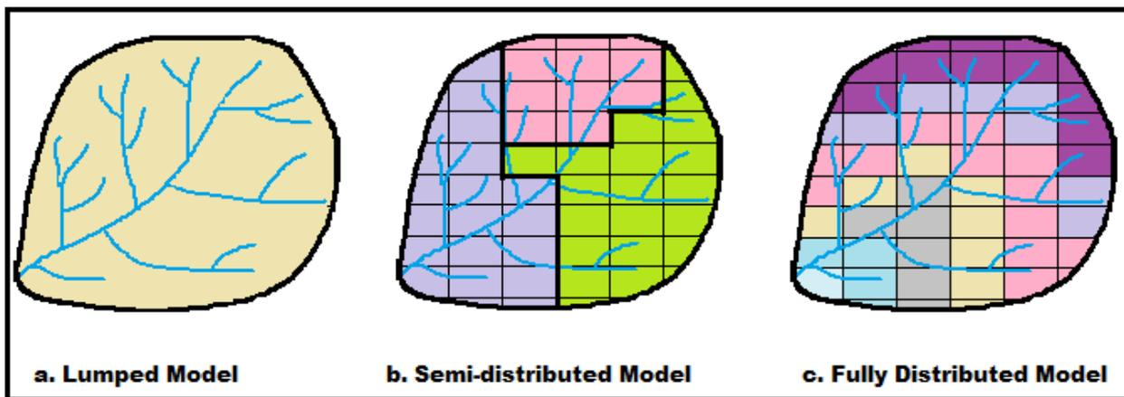
Figure 3.8. Spatial Scaling of Models at sub-basin level
