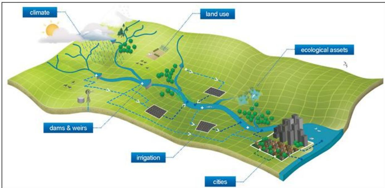
**Figure 6.2. A simplified sketch to highlight some of the aspects of eWater Source (eWater, 2015a)**
