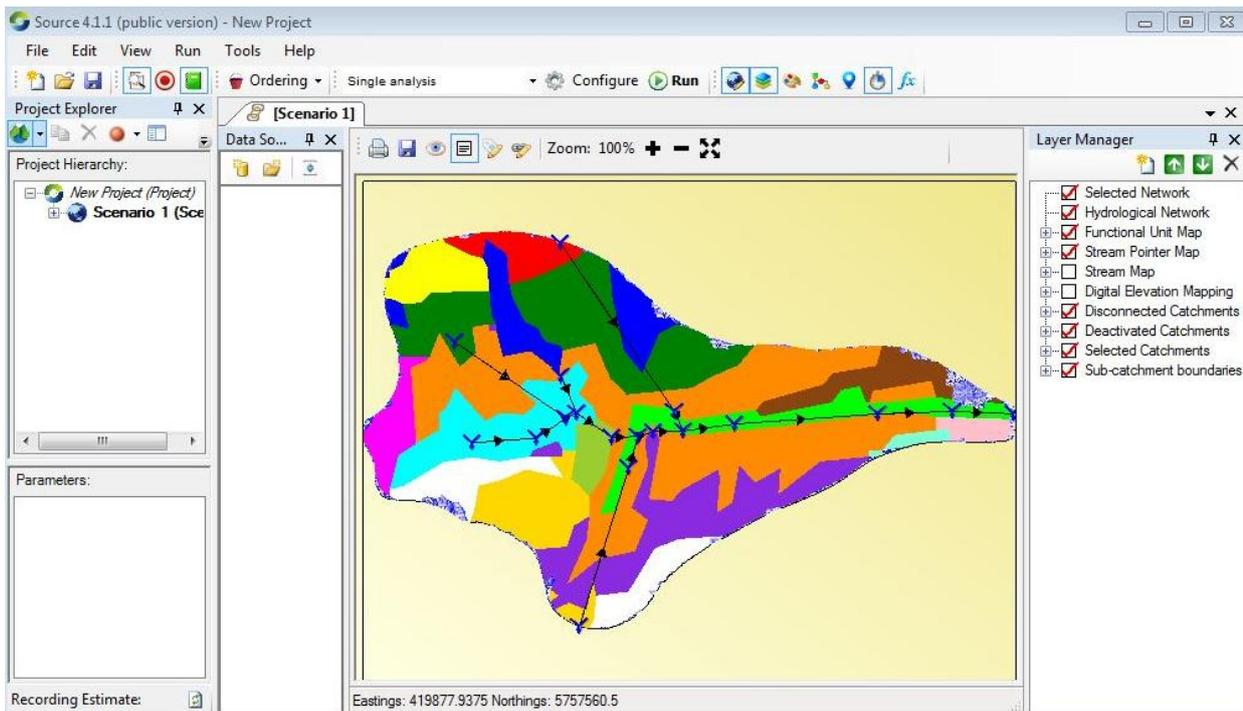
**Figure 6.7. The map with the Functional Units for every sub-catchment, in eWater**
