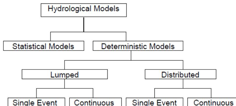
Figure 3.7. A simplified classification of hydrologic models (Bengtson and Padmanabhan, 1999)
