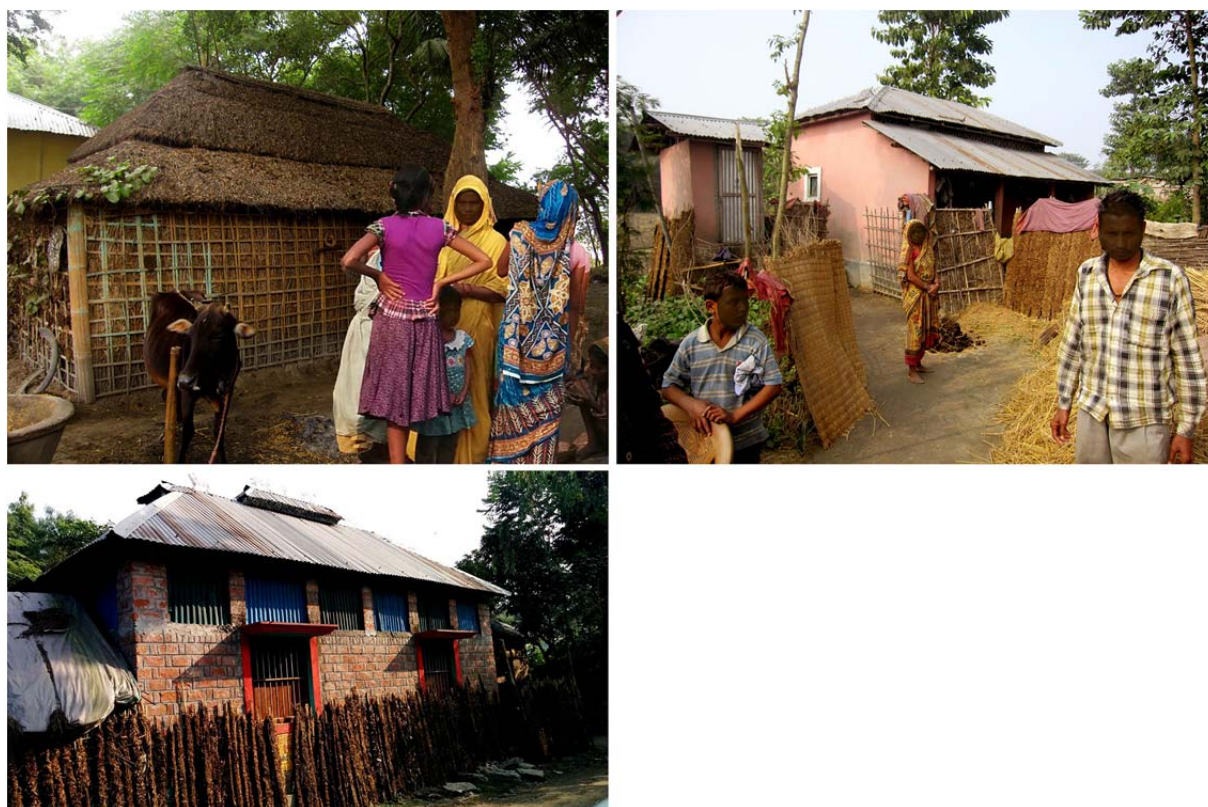
Figure 5: Top left - Photos of traditional bamboo and thatch house in Bihar; Top right – Improved bamboo houses in Orlaha and Bottom left – improvised brick houses in Puraini settlements after the 2008 Kosi River floods (source: author)
