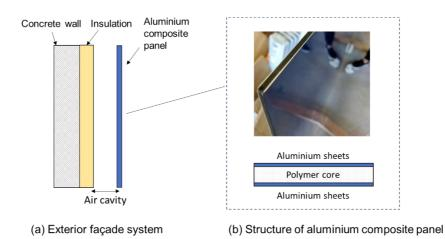
Figure 1: Diagram of (a) components of an exterior facade system and (b) the structure of the aluminium composite panel.
