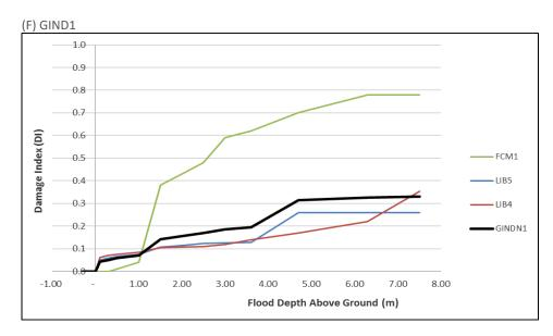
Figure 5: Flood Vulnerability functions: detailed and generalised (cont.).
