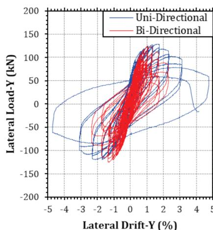
Figure 3: Load-drift behavior (uni-directional vs bi-directional)
