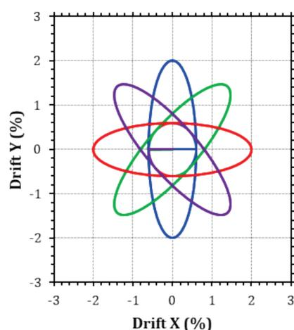
Figure 1: Proposed earthquake loading protocol
