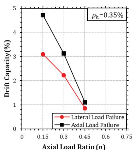
Figure 2: Reduction in drift capacity with axial load
