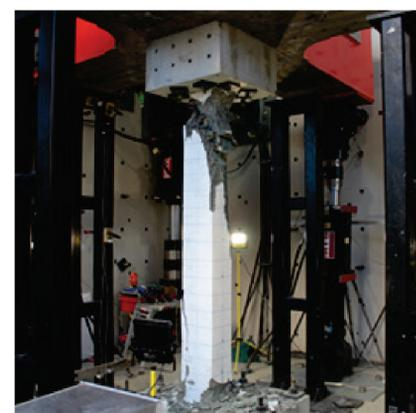
Figure 4: Column tested till collapse
