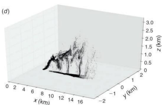
**Figure 2:** Snapshot of ember transport in the turbulent plume in Figure 1. The embers fall out in clumps as they experience weaker updrafts in the plume.
