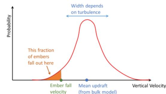
**Figure 5:** At each point along the plume, there is a probability distribution of updrafts. The width and mean of the distribution varies along the plume. The fraction of embers that fall out depends on probability (updraft < fall velocity).
