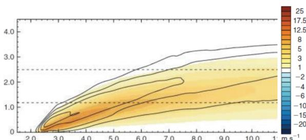
**Figure 4:** Mean plume updraft (colour) and turbulence intensity (contours, logarithmic scale) from the large-eddy model simulation.
