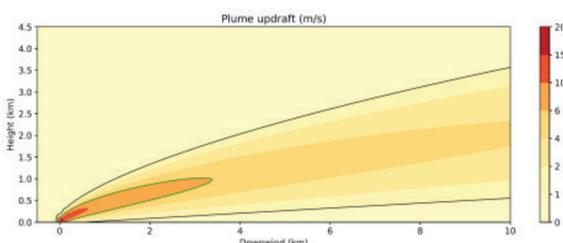
**Figure 3:** Simulated updraft from a bulk plume model. The green contour is 6 m/s updraft and indicates that part of the mean plume that can loft typical firebrands.
