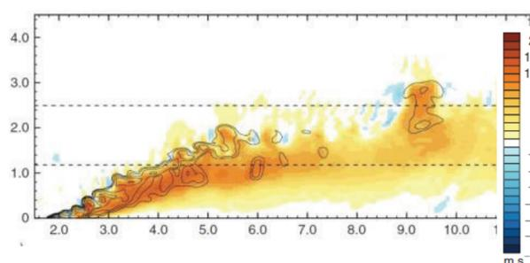
**Figure 1:** Large-eddy simulation of a turbulent bushfire plume. Shading shows the vertical velocity and contours the temperature perturbation.
