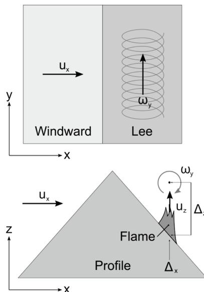
**Figure 2:** Schematic set-up of the near-field model.
