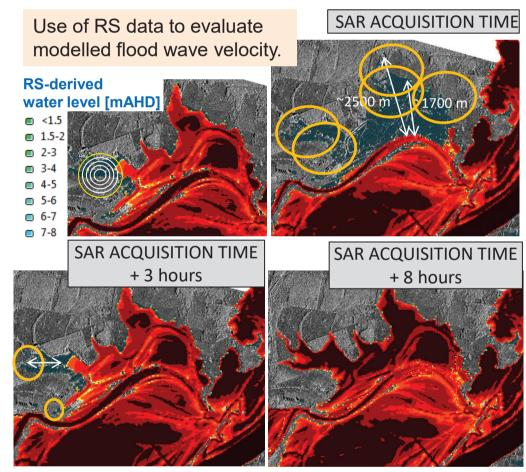
Fig 6 – RS-derived wet/dry boundary points at overpass time and modelled flood extent and depth at different times.
