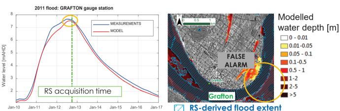
Fig 4 – Grafton: modelled and measured water level. Fig 5 – Grafton: modelled and RS-derived flood extent.
