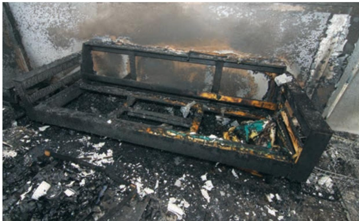
The room with no sprinkler and its synthetic, flammable contents were completely destroyed during the demonstration burn.
