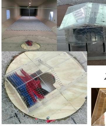
Tests in Wind Tunnel at the Cyclone Testing Station, James Cook University. On representative houses at a length scale  $(L_r)$  of 1/50
