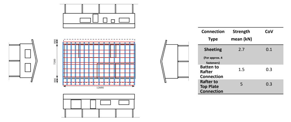
Failure when the load >strength: Failure Modes- Roof cladding: Batten-Rafter: Rafter-top plate:
