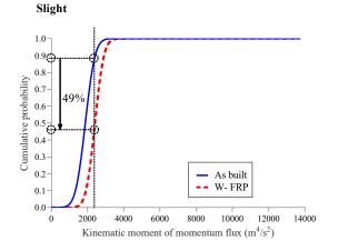
The reduction in probability of failure using FRP wraps is more pronounced at the extensive damage state (i.e. drifts at peak in capacity curves)
