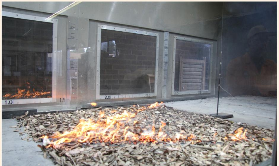
▲ Above: AN EXPERIMENTAL SEPARATED V-SHAPED FIRE CONDUCTED IN THE CSIRO PYROTRON. PHOTO: ANDREW SULLIVAN, CSIRO
