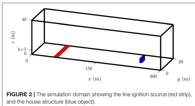
**FIGURE 2 |** The simulation domain showing the line ignition source (red strip), and the house structure (blue object).
