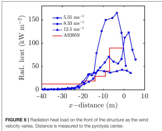
**FIGURE 6** | Radiation heat load on the front of the structure as the wind velocity varies. Distance is measured to the pyrolysis center.
