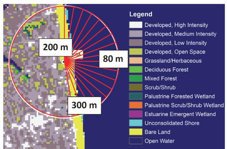
Figure 2: StickNet tower 103A deployed at the beach for Hurricane Sandy (2012). Coastal Change Analysis Program (C-CAP) land cover information on top including 10 degree fetch cones and distances.
