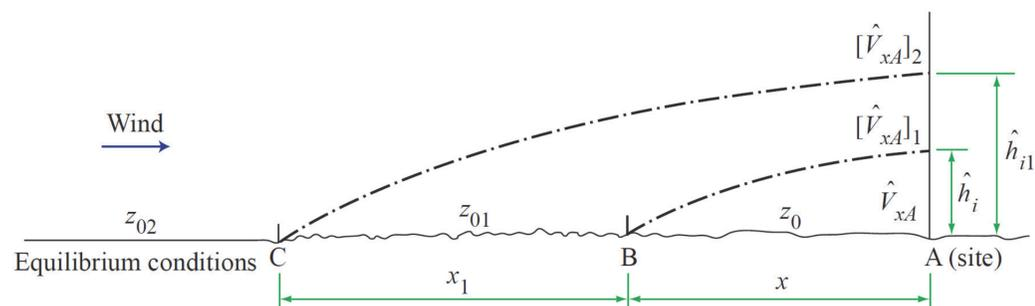
Figure 1: Two step changes in terrain roughness (ESDU 83045, 1983)
