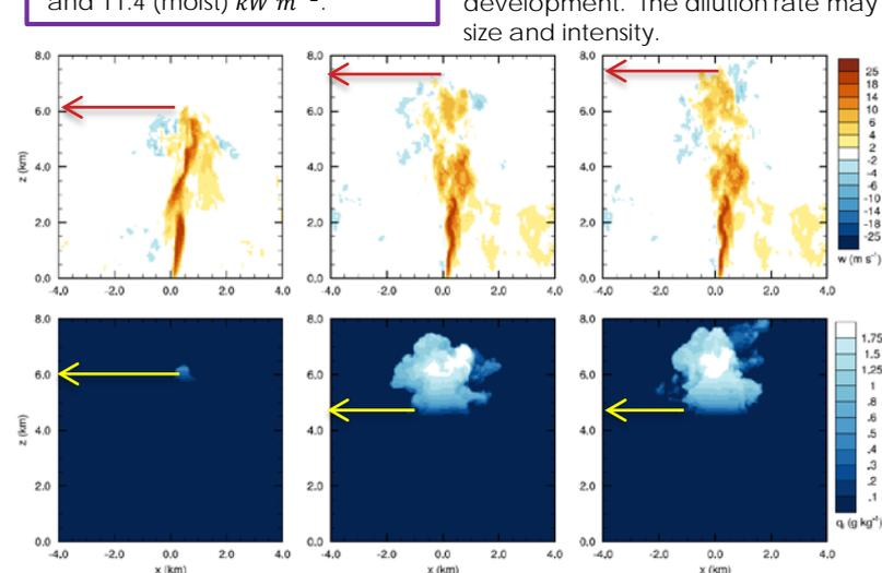
**Figure 2:** Vertical velocity (upper) and cloud water (lower) for the 2 (left) and 4 (centre) g kg<sup>-1</sup> boundary layer moisture simulations. The moist boundary layer (4 g kg<sup>-1</sup>) simulation is repeated with a moist fire (11.4 kW m<sup>-2</sup>, right). The arrows indicate cloud base (yellow) and plume top (red) height.
