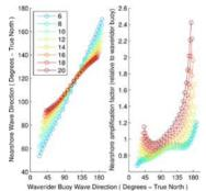
Summary of all SWAN wave model simulations for example nearshore location at Old Bar (see map to left) showing change in wave direction (left) and height (right) due to shoaling and refraction for wave periods ranging from 6-20 seconds. (# SWAN - Simulating WAves Nearshore) http://swanmodel.sourceforge.net/
