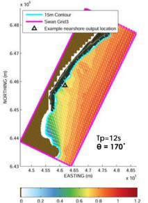
Example SWAN wave simulation for Grid 3 at Old Bar, showing direction (arrows) and ratio of nearshore wave height to height at waverider buoy. 15 m depth contour (blue) defines seaward boundary of sediment transport model.
