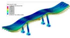
Considered damaged scenarios are a weakened girder to represent damage from debris impact; a longitudinal crack applied to the web of the girder to simulate damage from impact; a pier crack and pier scour.
