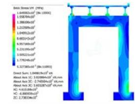
Load capacity based vulnerability index depends on the loads that caused the capacity of the bridge to be exceeded for both the damaged and undamaged state. Weakened girder case produces the highest vulnerability for all load combinations except for the traffic and hydrodynamic force load, where the pier crack gave the highest value of approximately 0.8
