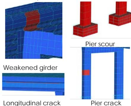
The areas of interest were those where the highest stresses were located and also where the damaged bridge sections were applied. The peak stress occurred with the ultimate impact load being applied directly to the section of weakened girder above the headstock.
