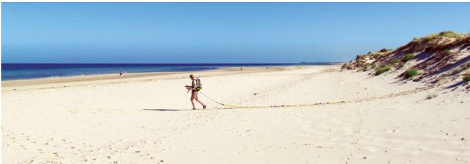
▲ **Above:** A RESEARCHER USES A GROUND PENETRATING RADAR DEVICE AT OLD BAR BEACH IN NSW TO UNDERSTAND HOW THE BEACH WILL REACT TO A STORM. PHOTO: GEOSCIENCE AUSTRALIA
