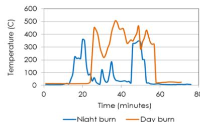
Figure 5. Surface temperatures of simulated fire fronts coincident to satellite overpass times.
