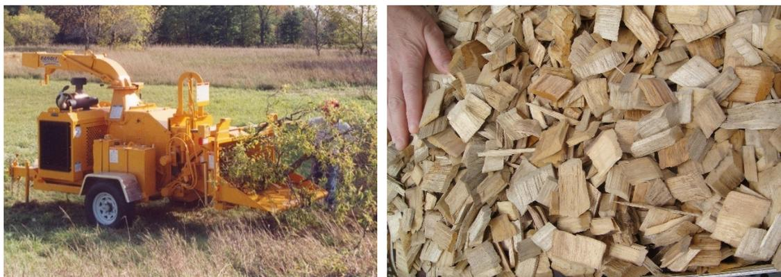
FIGURE 10. WOOD CHIPPER AND WOOD CHIPS. SOURCE: WIKIPEDIA
