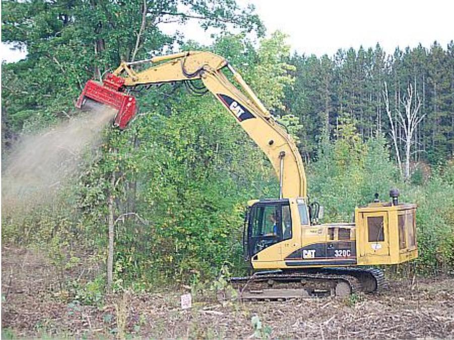
FIGURE 5. EXAMPLE OF MULCHING TREATMENT. SOURCE: WIKIMEDIA COMMONS (2013)
